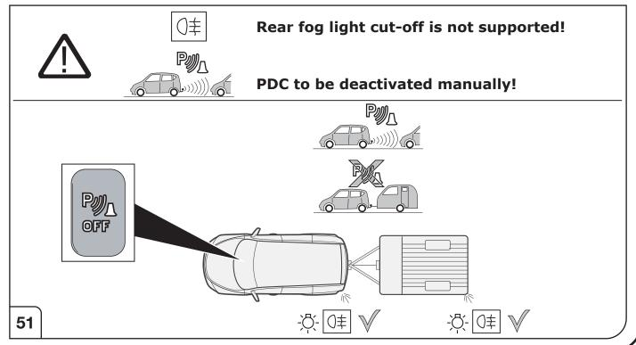
The following light functions for the trailer are **not supported** by all towing vehicles **with DRL circuit:**
